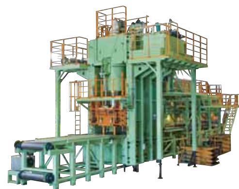
Filter molding press (Production of external wall material etc.)
